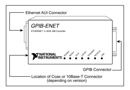
Figure 1-1. GPIB-ENET Top Panel
